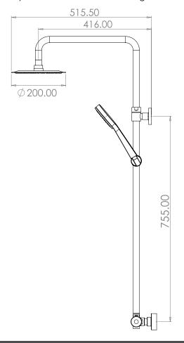
Riser rail adjustment - MIN 765mm MAX 1165mm.
