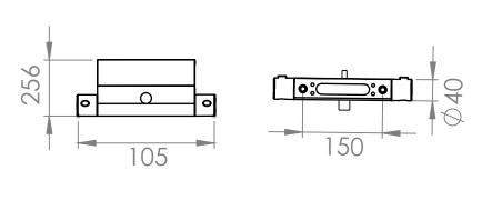
Riser rail adjustment - MIN 765mm MAX 1165mm.
