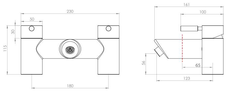
SHOWER HOSE AND DIVERTER POSITIONED 65MM FROM PIPE CENTRES, SHOWN IN RED ON DIAGRAM.
